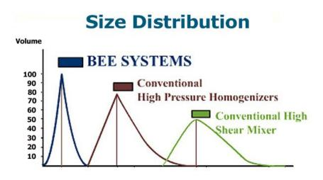
BEE International High Pressure Homogenizers for a tight distribution of smaller particles
